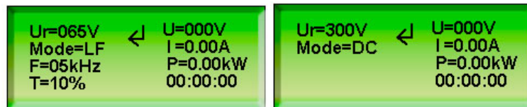
Pic.3 LCD display at the work mode, impulse (right) and DC mode (left)
