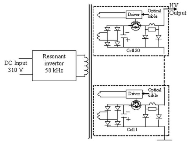
FIG. 4. Simplified schematic of the cellular high voltage approach adopted here.
