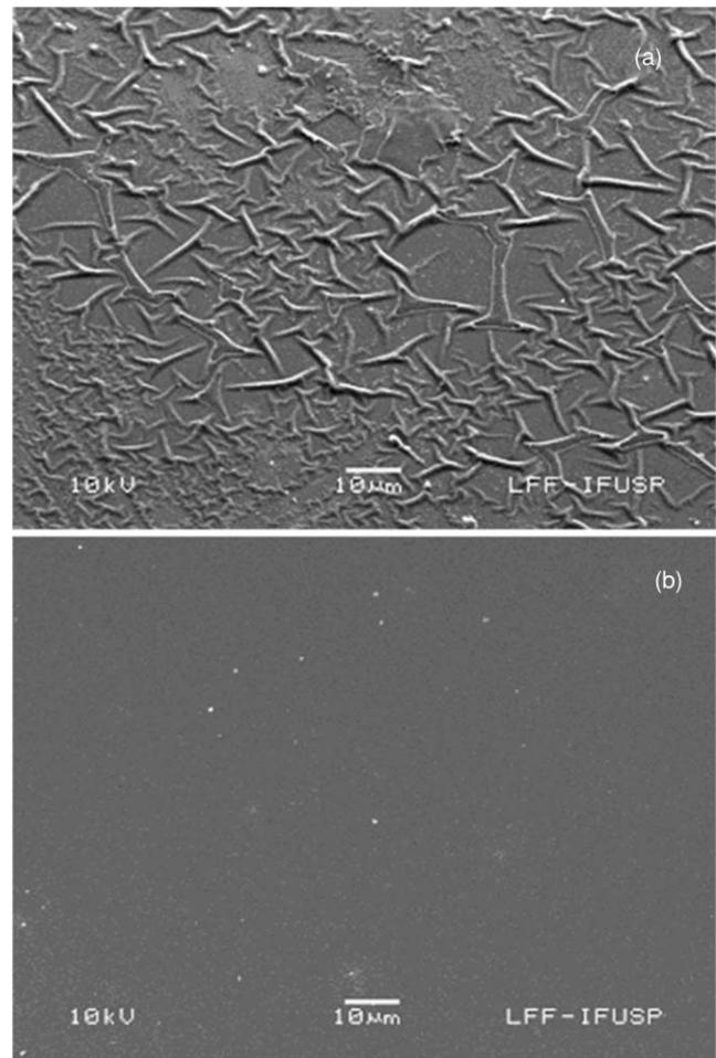
FIG. 5. SEM micrographs of DLC films formed with and without interface mixing: (a) no mixing; (b) with mixing as produced by 5 keV  $C^+$  ion implantation prior to the DLC deposition. In both cases the DLC deposition was carried out with pulsed substrate bias of –100 V so as to maximize the  $sp^3$ -bonded carbon atom fraction in the film, and so also the film internal stress.
