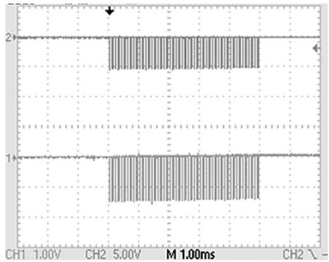
FIG. 3. Oscilloscope showing the 5 ms long gated pulse packet.  $700 \Omega$  resistive load. Upper trace: voltage (1 kV/cm), lower trace: current (1 A/cm), sweep speed 1 ms/cm
